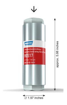
WITT Automatic Quick Acting Shut-Off Devices (slam shut valves) for reliable protection against dangerous decomposition of acetylene in high pressure pipelines in accordance to EN ISO 14114.
