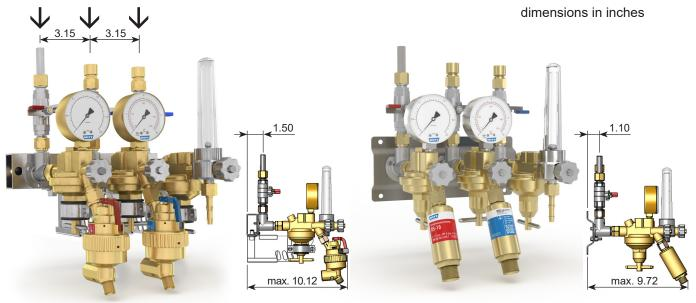
Outlet points easy to use for withdrawal of technical gases. To mount on wall for connection with a central gas supply system (ring line). The compact design is modular expansible and offers a variety of possible combinations.
