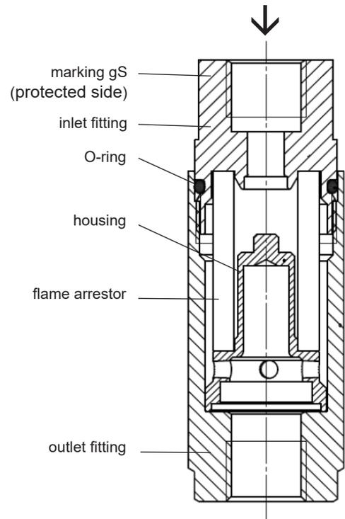
The deflagration volume protection device is ideal for protection of plants and equipment with a volume of max. 4.6 l.
