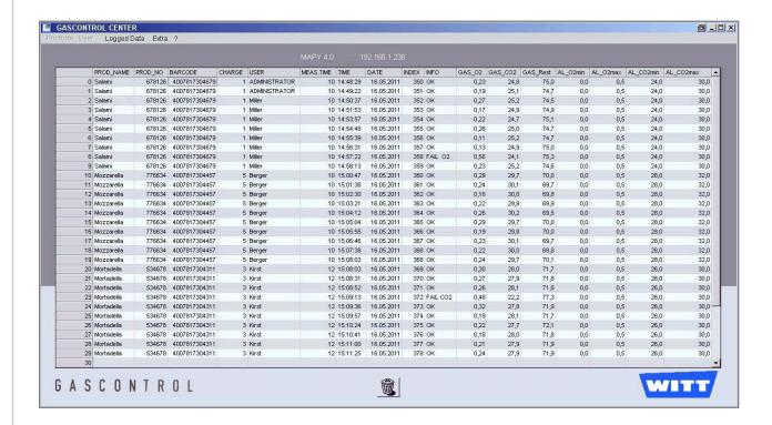
Windows-Software for the documentation of analysis-results of MAPY, LEAK-MASTER®, MAPMAX and other WITT- equipment with integrated or separate analysis.
