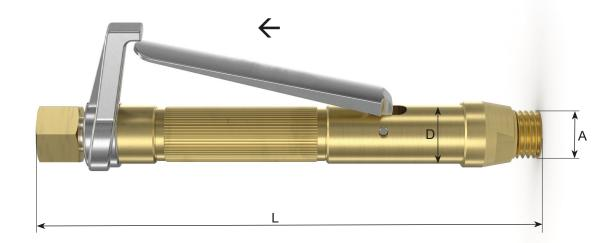
Lever valve for automatic stop of gas supply by releasing. Adjusting the oxygen supply with lever valve. The gas supply will be closed by loosing the lever and guarantees a high degree of safety.
