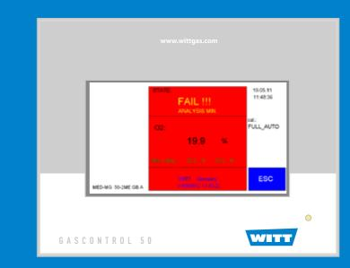
> PARALLEL CONTROL SYSTEMS WITH SELF MONITORING The mixing system works with 2 parallel control units and one independent alarm module. A continuous monitoring ensures the error-free operation of the three safety components. The control units and the alarm module are monitored by each other (handshake concept).
