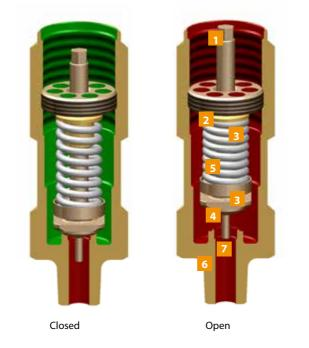
Valve piston Screwing ring Spring retainer Valve seal **Compression spring** Housing
